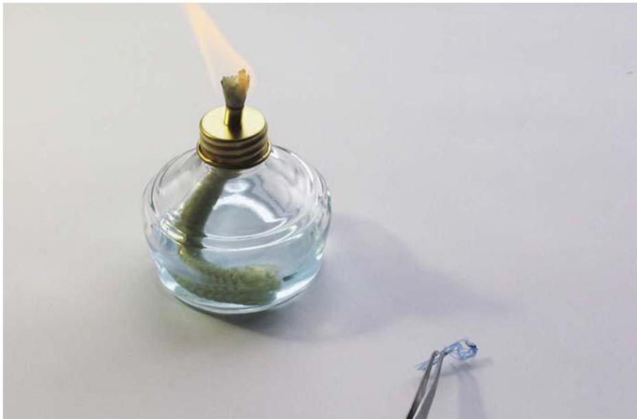
Picture 6. A yarn when is removed from the flame.
